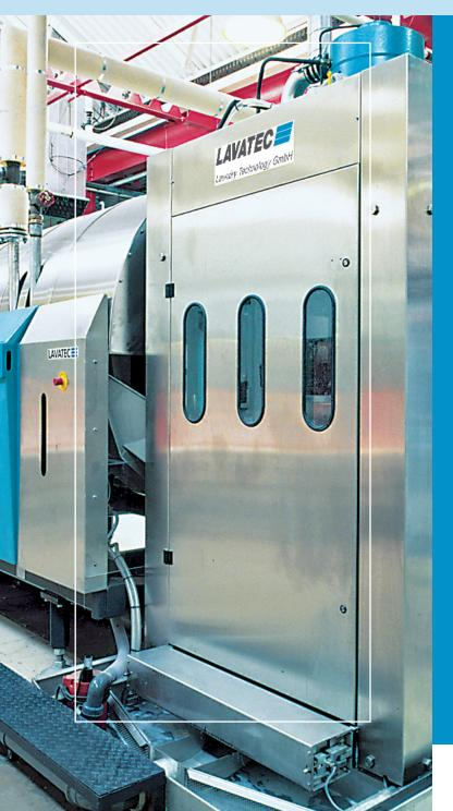
"The Lavatec Water Extraction Press ensures that the dryers downstream need to vaporize smaller amounts of water."
